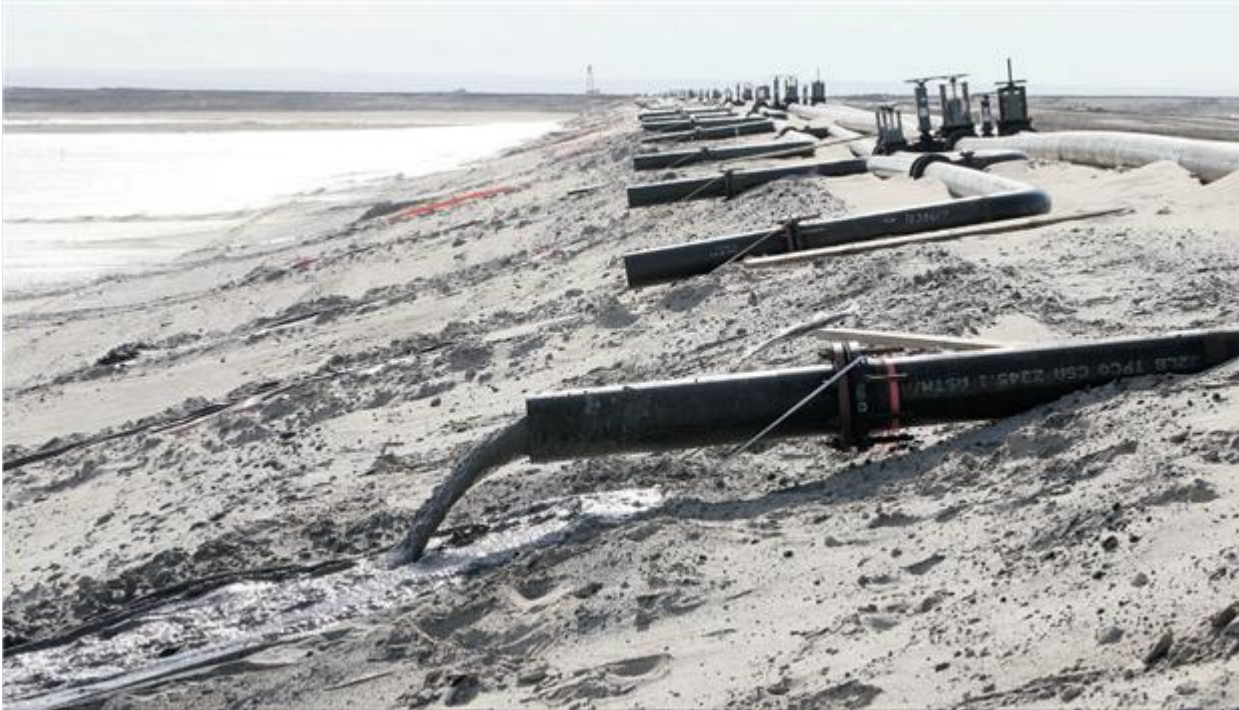
Figure 4-8: Example of multiple thickened tailings discharge outlets in the summer on level ground in Fort McMurray, Alberta. (Photograph by Rick MacWilliam, Edmonton Journal)
